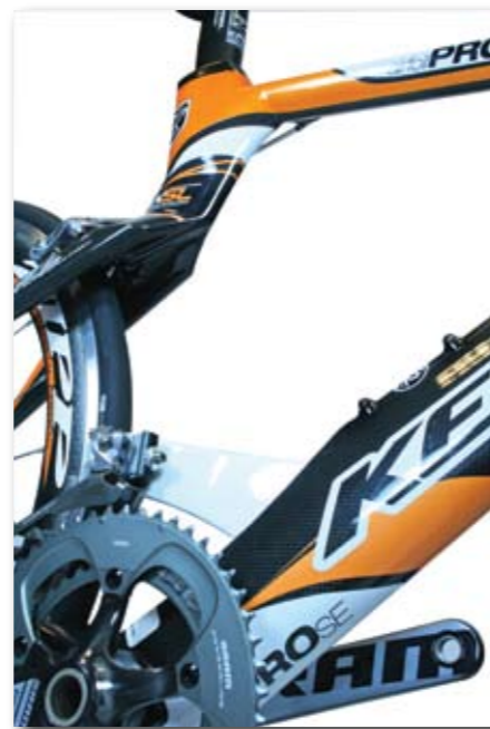
LOOK ODD?: No seat tube – the Kestrel approach
